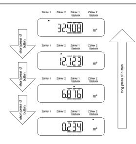
The LCD of the pulse adapter has 4 display levels:
