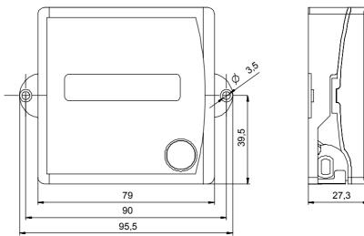
Dimensions in mm Connecting cable length is 350 mm.
